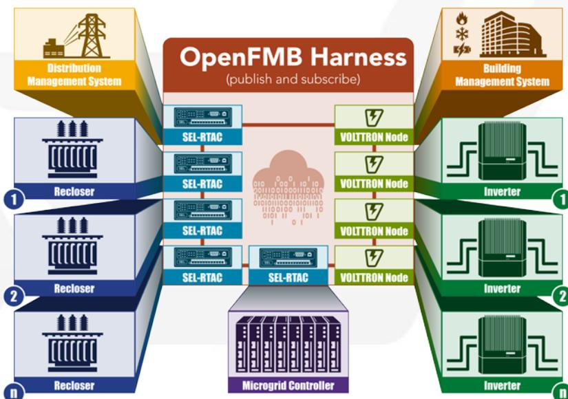
A segmented, self-healing distribution system uses decentralized assets and forms microgrids to isolate disruptions and minimize outages. It uses distributed energy resources such as solar inverters, smart loads such as building management systems, utility switching devices such as reclosers, and distribution management systems, all controlled locally by a microgrid controller through the open FMB harness.
