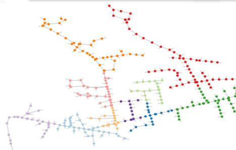
Circuit reduction results showing a reduced feeder model with ~10 representative nodes. Performed K-means clustering using electrical distances in combination with voltage data from QSTS model
