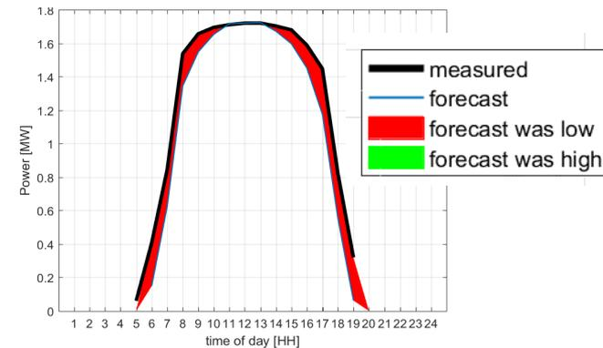
Added PV capacity makes substation forecast low
